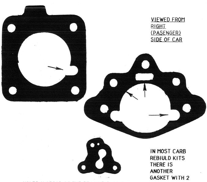
HOLES INSTEAD OF THE STOCK FIGURE 8 HOLE FOR THE AIR BLEED VALVE. USE THE ONE WITH 2 HOLES.
