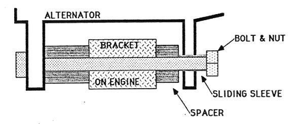
When the long mounting bolt for the alternator is removed this piece can fall out without being noticed because it is below the alternator and out of sight. Two things can then happen. First the mounting bolt/nut can be tightened until the rear, front, or both mounts on the alternator break off. Or, the alternator moves fore and aft until something gives (the belt catches and breaks, the adjustment mount breaks, etc.).
